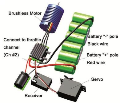
2.1 Turn on the transmitter, set the "EPA/ATV" value of throttle channel to "100%", and disable the "ABS" brake function of your transmitter if it does has this function. If you are using a Futaba transmitter, please set the direction of the throttle channel to "REV"
