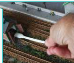
At intervals the swab may need cleaning. To clean swab apply a little solvent and blot dry with clean tissue.
