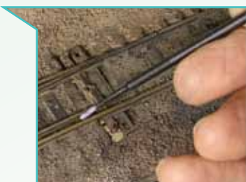
Using the brush with a little Track Magic to clean points contacts.
