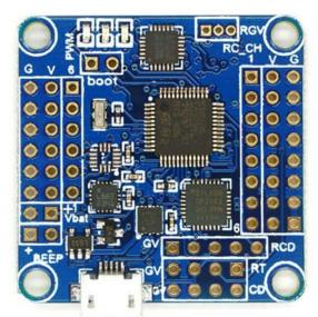
The difference between 10dof and 6 dof version are compass and barometer, the 6 dof version HASN'T HMC5883I and MS5611.
