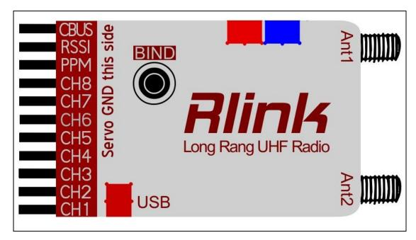
The Rlink rx is more or less the same as normal 2.4G receivers, but the diversity antennas are connected with SMA connectors, recommend to set up as "V" shape in your aircraft, and make sure the antennas have no touch with any metal, carbon or any other conductive object. When the rx is connected with too many servos or the servos are too big and draw too much current, you need to use a separated UBEC to power the Rlink
