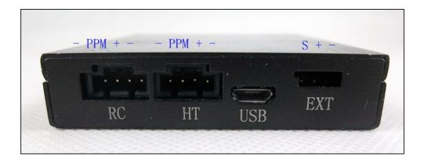
As above shows, the Tx module support 2 PPM signals input with 4-pin Molex connectors(the pins' definition are as above), the 2 PPM sources could be radio or head-tracker or any other PPM generator. The 2 PPM source could be merged into 1 PPM output with 16 channels at most.
