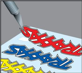
To apply the decals, place one end down, hold the other end up, and gradually smooth the decal down with your finger as you go. This will prevent air bubbles. Placing both ends of the decal down and then trying to smooth it out will result in air pockets. Look at the photos on the box for typical decal placement.
