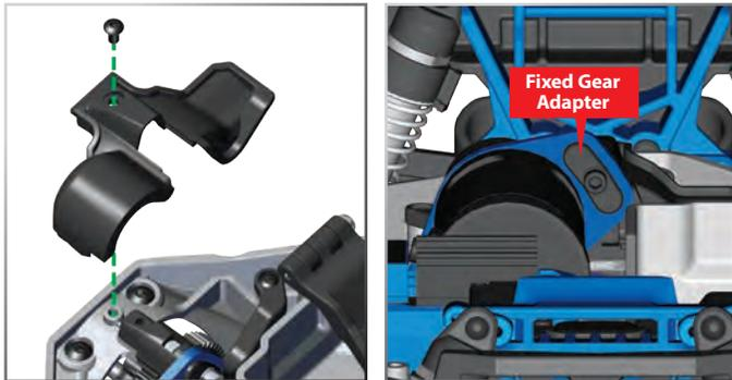
If you choose to do so, you can also set the gear mesh manually without using the fixed gear adapter. With the adapter removed, loosen the motor screw. Cut a narrow strip of notebook paper and run it into the gear mesh. Slide the motor and pinion gear into the spur gear. Retighten the motor screw, and then remove the strip of paper. You should be able to run a fresh strip of paper through the gears without binding them.
