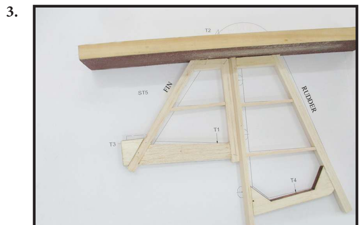
2. Cut off the excess balsa wood part and sanding smooth and flat the edge. (Photo 3).
