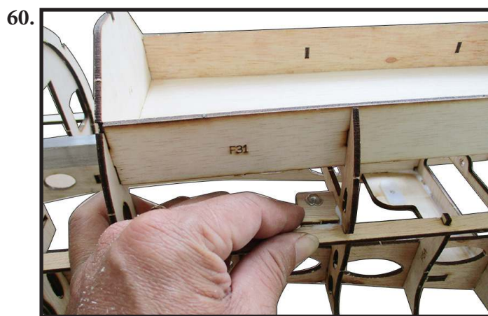
Locate and assemble FS5 (servo mount) as (photo 61).
