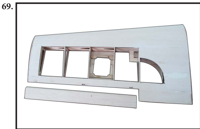
Locate and sawn the slot for hinge. Note: cut off the slot fit so that avoid so wide cause CA hinge will fall out. (Photo 70).
