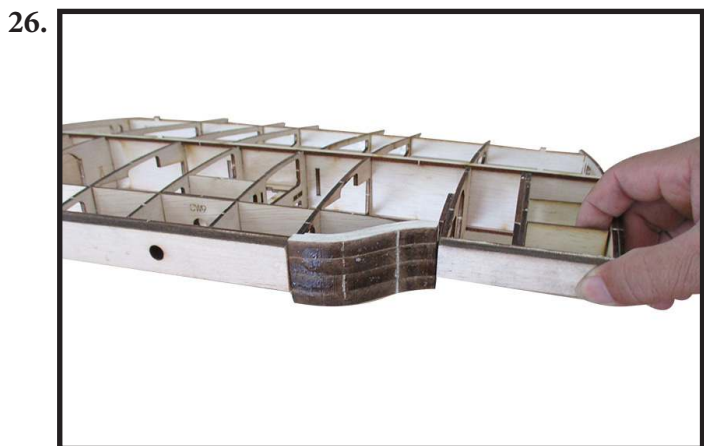
Cut off excess part of balsa and sanding for leading edge look like seamless. (Photo 27,28).
