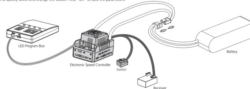
The program box needs to be connected to the independent programming port for 10BL120 G2, and fan port for 8BL150 G2. Otherwise, it will not work!
