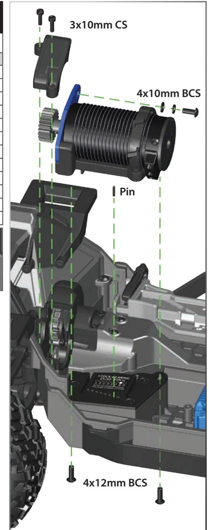
**Note:** Should you choose to do so, you can also set the gear mesh manually without the pin. With the pin removed, use the two 4x12mm button-head cap screws on the bottom of the chassis to set gear mesh. Loosen the two 4x12mm button-head cap screws.
