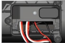
**Note:** For best performance, it is recommended that the receiver be installed in the original orientation as shown.
