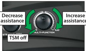
When driving on surfaces with some traction, decrease the TSM setting to allow the vehicle to feel more “loose” for power sliding, drifting, and so on. On surfaces with very little traction (loose dirt, smooth concrete, ice/snow), increase TSM to maximize acceleration and control.
