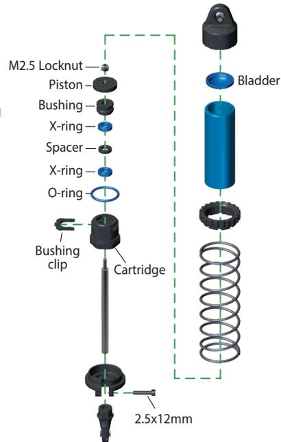
3. Remove the M2.5 locknut, piston, 2.5x5mm washer, and the existing cartridge assembly from the shock shaft.
