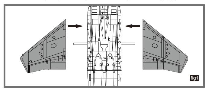
3. Secure the left and right wing to the fuselage using the 4 screws included (fig2)
