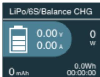
On the main interface, hold the ENTER
