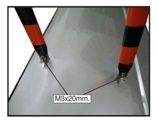
3) Repeat steps to prepare the remaining wing panel for installation and use pliers to bend four of the brass tabs at a slight angle.Make the bend slightly biased toward the larger hole in the tab.
