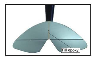
3) Slide the vertical stabilizer back in place. Using a triangle, check to ensure that the vertical stabilizer is aligned 90° to the horizontal stabilizer.
