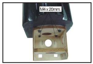
3) Attach the motor to the front of the electric motor box using four 4mm blind nut, four M3x15mm hex head bolts to secure the motor. Please see picture shown.
