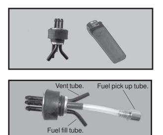
$\square$  3) Carefully bend the second nylon tube up at a 45° angle. This tube is the vent tube.
