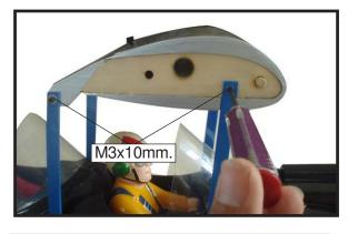
ATTACHMENT WING-FUSELAGE. Attach the aluminium tube into fuselage.
