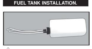
You should mark which tube is the vent and which is the fuel pickup when you attach fuel tubing to the tubes in the stopper. Once the tank is installed inside the fuselage, it may be difficult to determine which is which.  $\Box$  7) Slide the fuel tank into the fuselage. Guide the lines from the tank through the hole in the firewall.
