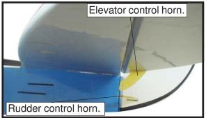
$\Box$  3) Thread one clevis and M3 lock nut on to each elevator control rod. Thread the horns on until they are flush with the ends of the control rods.
