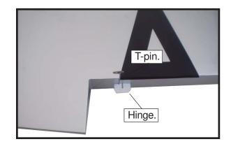
□ 3) Slide the aileron on the wing panel until there is only a slight gap. The hinge is now centered on the wing panel and aileron. Remove the T-pins and snug the aileron against the wing panel. A gap of 1/64" or less should be maintained between the wing panel and aileron.
