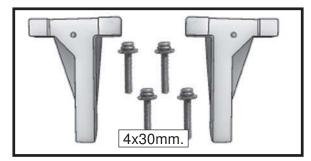
2) Use four 4x30mm head bolts and four 4mm washers to attach the engine mount rails to the firewall. Tighten the screws . Make sure to use threadlock on the screws to help prevent them from vibrating loose.
