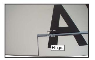
□ 4) Deflect the aileron and completely saturate each hinge with thin C/A glue. The ailerons front surface should lightly contact the wing during this procedure. Ideally, when the hinges are glued in place, a 1/64" gap or less will be maintained throughout the lengh of the aileron to the wing panel hinge line.
