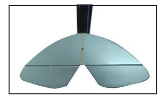
$\Box$  4) With the stabilizer held firmly in place, use a pen and draw lines onto the stabilizer where it and the fuselage sides meet. Do this on both the right and left sides and top and bottom of the stabilizer.
