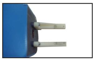
4) On the fire wall has the location for the throttle pusshrod tube (pre-drill).
