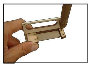
4) Apply 2-3 drops of thin C/A to each of the mounting holes. Allow the C/A to cure without using accelerator.
