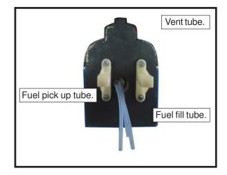
9) Connect the lines from the tank to the engine and muffler. The vent line will connect to the muffler and the line from the clunk to the carburetor. Blow through one of the lines to ensure the fuel lines have not become kinked inside the fuel tank compartment. Air should flow through easily.
