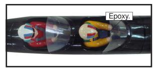
4) Position the canopy onto the fuselage. Trace around the canopy and onto the fuselage using a felt-tipped pen.
