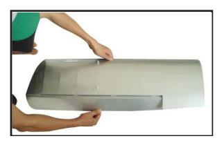
$\Box$  5) Turn the wing panel over and deflect the aileron in the opposite direction from the opposite side. Apply thin C/A glue to each hinge, making sure that the C/A penetrates into both the aileron and wing panel.
