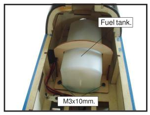
$\square$  8) Use plywood template to hold in place the fuel tank with C/A glue to secure the fuel tank inside the fuselage.
