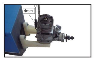
3) Use a drill to drill the four holes in the engine mount rails.
