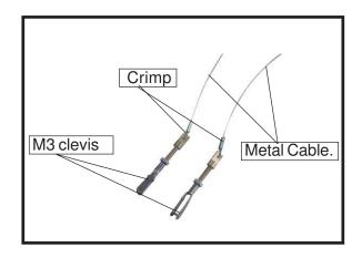
2) Attach the clevis to the brass tab next to the rear interplane strut on the upper-lower wing.Slide a copper crimp on the cable. Pass the cable through the brass tab on the upper wing, the back through the copper crimp.
