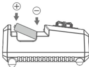
Inserting AAA Batteries
