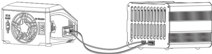
3. Connect the battery to D200neo on Port A;
