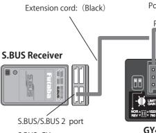
S.BUS CH Rudder --- 4CH Gyro gain --- 5CH
