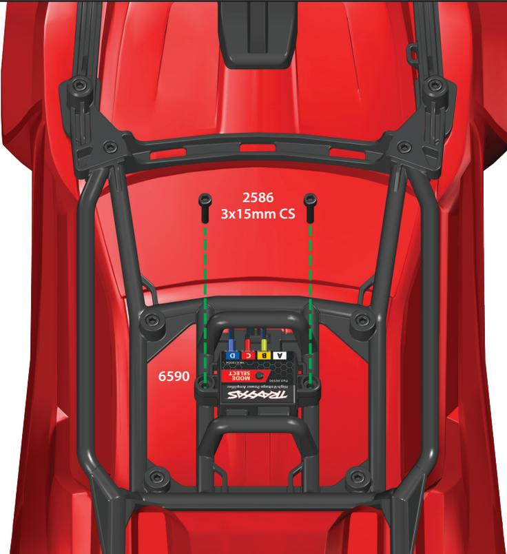
Turn the body over (viewing the underside) and fasten the high-voltage power amplifier to the body cage using the included 3x15mm cap screws (2). Position the amplifier so that the 4 lighting connection ports point to the front of the body. Plug the 4 LED harness connectors into the power amplifier, matching the colors on the wires with the corresponding colors on the amplifier ports (white, yellow, red, blue).
