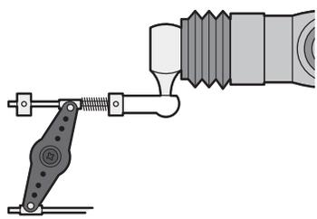
Adjust the throttle servo so that unreasonable force is not applied when the engine carburetor is fully open, fully closed, and the brakes are applied fully.
