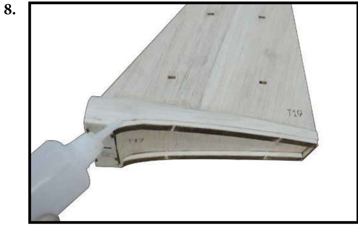
- Attach 8mm balsa block for two side by CA glue as photo.
