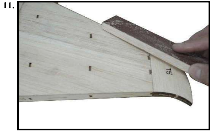
- Use sandpaper bar for sanding the surface of rudder.
