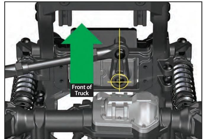
If you are using aftermarket servos, it is important to use servo horns designed for TRX-4. The servo horns must measure 22mm from the steering linkage mounting hole to the servo mounting hole.
