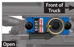
**Differential Locked:** Switch the transmitter and receiver on. Move the T-Lock switch to the forward-most position to lock the rear differential. Confirm that the servo's output shaft turns counterclockwise to rotate the servo horn to the position shown.
