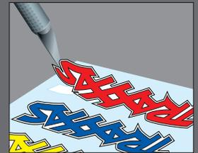
To apply the decals, place one end down, hold the other end up, and gradually smooth the decal down with your finger as you go. This will prevent air bubbles. Placing both ends of the decal down and then trying to smooth it out will result in air pockets. Look at the photos on the box for typical decal placement.
