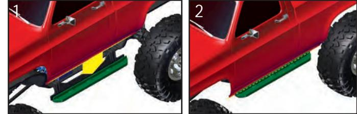
2. Press down on the body at each latch location until the latches snap into place.
