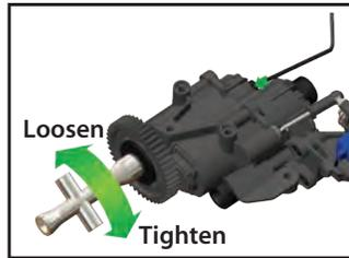
To restore factory settings, use the included 4-way wrench to turn the adjustment nut until all four spring washers are flat; then, tighten the nut an additional 1/16 turn (or until the slipper clutch does not allow the spur gear to slip during normal operation).
