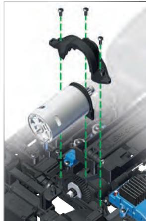
To set the gear mesh, use the chart to the left to identify the screw positions on the motor plate (A - H) that correspond with the chosen motor pinion (9-T - 22-T) and spur gear size (39-T or 45-T). Remove the two screws from the motor/motor plate and reinstall in the corresponding positions; reinstall the motor/motor plate assembly in the chassis.
