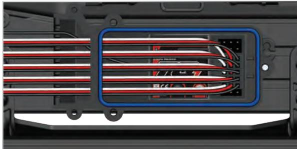
4. Apply a bead of silicone grease (Traxxas part #1647) to the wire clamp.
