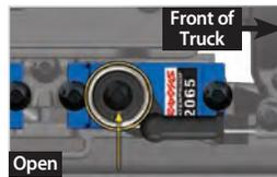
**Differential Locked:** Switch the transmitter and receiver on. Move the T-Lock switch to the middle position to lock the front differential. Confirm that the servo's output shaft turns counterclockwise to rotate the servo horn to the position shown.
