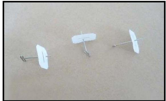
Remove each hinge from the wing panel and aileron and place a T-pin in the center of each hinge. Slide each hinge into the wing panel until the T-pin is snug against the wing panel. This will help ensure an equal amount of hinge is on either side of the hinge line when the aileron is mounted to the aileron.
