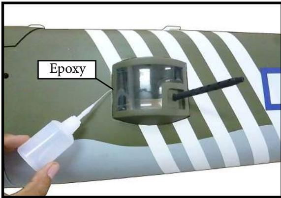
**STABILIZER INSTALLATION INTO FUSELAGE**
