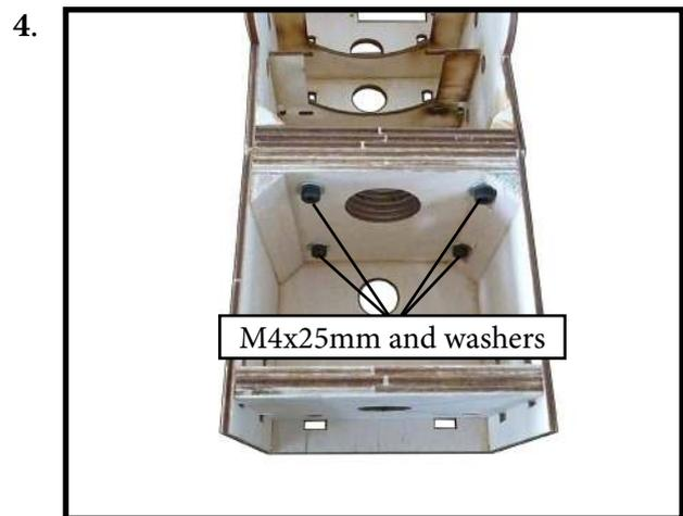
Attach the motor to the front of the electric motor box using four 4mm blind nut, four M4x25 mm hex head bolts to secure the motor. Please see picture shown.
