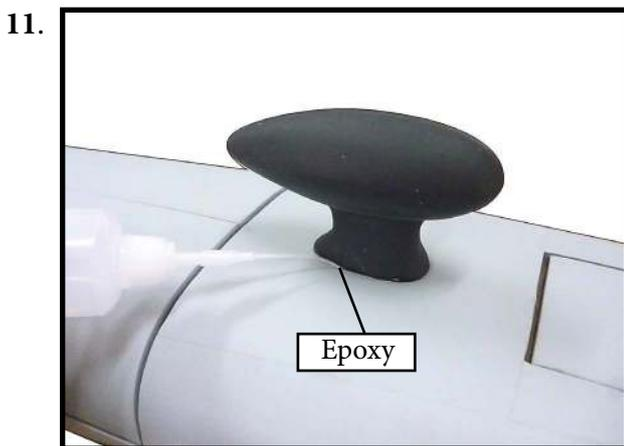
**GUN INSTALLATION TWO SIDE OF FUSelage**
