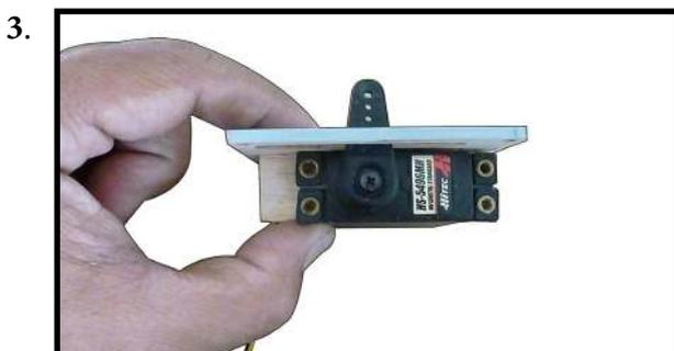
Use drill bit in a pin vise to drill the mouting holes in the blocks.
