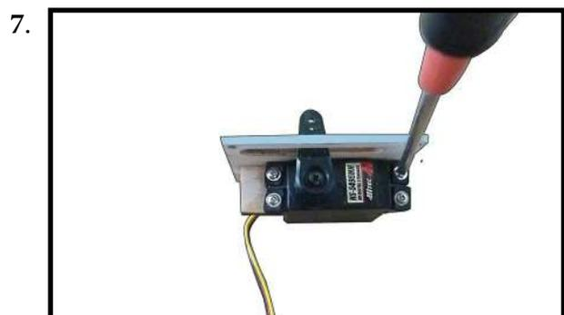
Apply 1-2 drops of thin C/A to each of the mounting tabs. Allow the C/A to cure without using accelerator.
