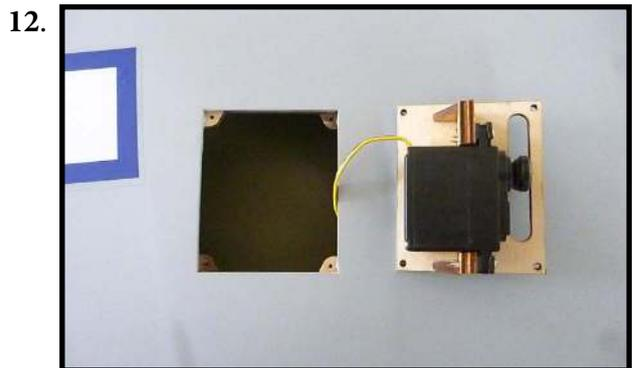
Set the aileron hatch in place and use a Phillips screw driver to install it with four wood screws.
