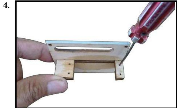
Apply 2-3 drops of thin C/A to each of the mounting holes. Allow the C/A to cure without using accelerator.
