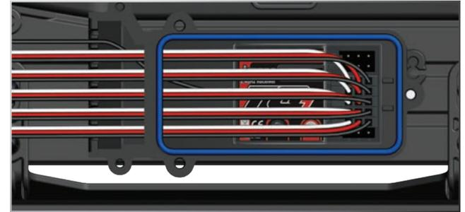
4. Apply a bead of silicone grease (Traxxas part #1647) to the wire clamp.
