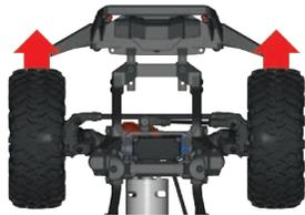
7. Gently operate the throttle trigger to ensure that you have forward and reverse operation, and that the motor stops when the throttle trigger is at neutral. **WARNING: Do not apply full throttle in forward or reverse while the model is elevated.**
