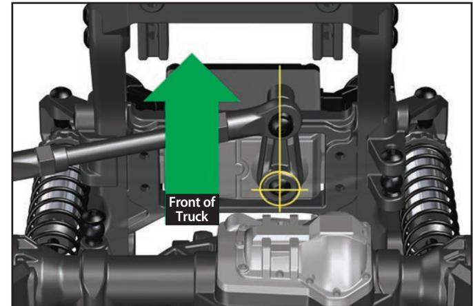
If you are using aftermarket servos, it is important to use servo horns designed for TRX-4 Sport. The servo horns must measure 22mm from the steering linkage mounting hole to the servo mounting hole.
