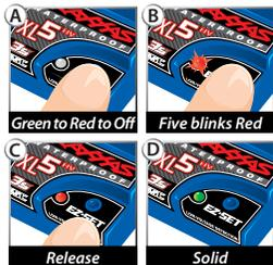
**Note:** If you missed the mode you wanted, keep the EZ-Set button pressed down and the blink cycle will repeat until the button is released and a Mode is selected.
