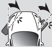
Blinking of the LED 4 times indicates that the gyro is in the limit setting mode. When the button switch is pressed once, the gyro enters the single-side (PWM signal wide side) setting mode.
