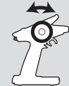
The servo automatically moves to the current limit position.
