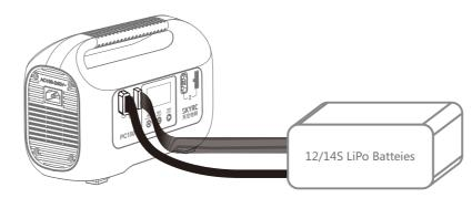
5) Select the Charge Mode: Fast Charge or Charge to long-press the START button for three seconds to start charging. Note: 12S and 14S batteries cannot be charged simultaneously; short-press the START button to stop charging or exit the abnormal state.
