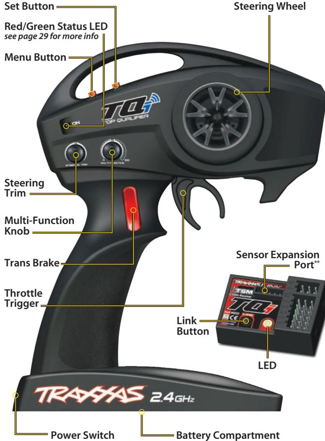
\*\*Accessory sensor port for use with the Telemetry Expander Module (see Traxxas.com for more information).
