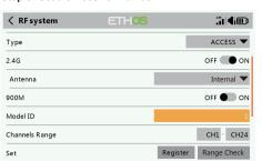
The system will assign you the receiver a number automatically, when you create a new model, and this can be easily changed. The range of the Model ID is 00-63, with the default number being 01. Once the receiver is set to the desired number and is bound to the TANDEM X20, the bind procedure will not need to be repeated unless the receiver number is changed. At this point, set the receiving number to your preferred number and repeat the binding operation.
