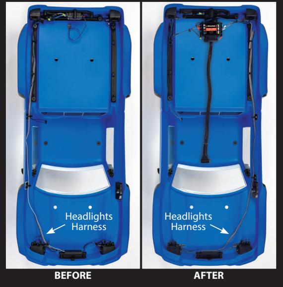
• If the 8085 LED light kit has already been installed, it will be necessary to remove the existing distribution block and mount in the body and install the new Pro Scale Lighting Distribution Block (part #6593, included with part #6591) using the new distribution block mount supplied with this kit. These instructions assume the 8085 LED Light Kit has already been installed.
