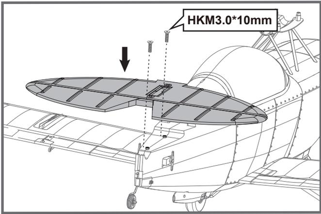
2. Align the vertical stabilizer with the horizontal stabilizer and push the surface down and forward until it is held securely in place.
