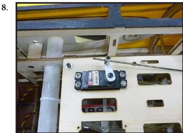
Move the throttle stick to the closed position and move the carburetor to closed. Use a 2.5mm hex wrench to tighten the screw that secures the throttle pushrod wire. Make sure to use threadlock on the screw so it does not vibrate loose.
