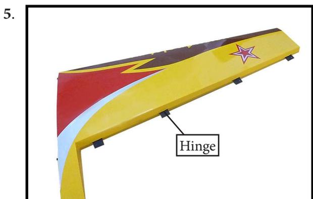
Press the aileron and wing together such that less than a 1/64" hinge line gap exists between the aileron and wing. The bevels should virtually touch. Use a paper towel and rubbing alcohol to wipe away any visible epoxy around the hinges.
