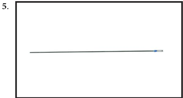
Attach throttle pushrod to the carburetor throttle arm with the ball link.
