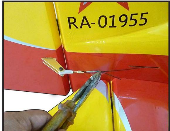
Cut off excess cable as shown.
