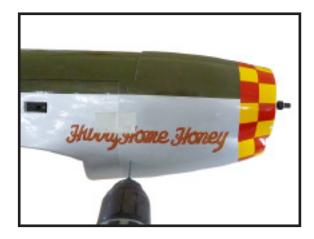
3) Tape a piece of card stock to the fuselage to indicate the location of the mufflr, needle valve, and any other items that may require access when the cowl is mounted. Slide the cowl on the fuselage, and transfer these locations onto the cowl. Use a drill, rotary tool and sanding drum to make any cut-outs in the cowl before securing it to the fuselage.
