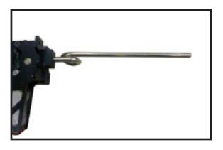
4) Fit the retract into the wing. Mark the locations for the retract mounting screws. Next, use a drill and drill bit to drill the holes for the screws.
