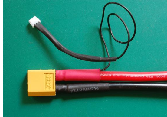
Figure B-2B: Main Power Lead
