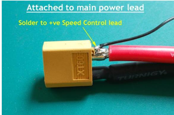
Figure B-1A: Main Power Lead
