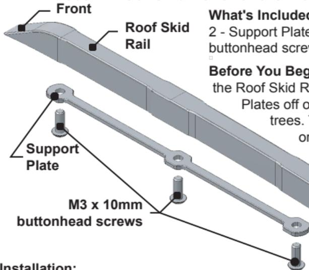
**What's Included:** 2 - Roof Skid Rails, 2 - Support Plates, 6 - M3 x 10mm buttonhead screws. □
