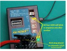
To complete the reset, you may wish to set the stabilizer pots back to the 12 o'clock position and return all DIP switches to OFF, but this is not required.
