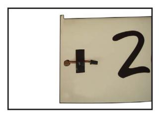
3) Set the aileron hatch in place and use a Phillips screw driver to install it with four wood screws.
