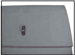
☐ 2)Secure the servos with the screws provided with your radio system.
