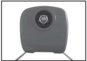
Slide the fiberglass cowl over the engine and line up the back edge of the cowl with the marks you made on the fuselage then trim and cut.
