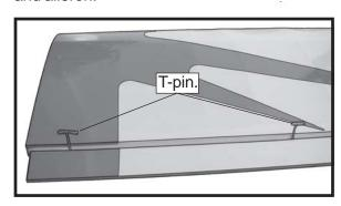
□ 4)Deflect the aileron and completely saturate each hinge with thin C/A glue. The ailerons front surface should lightly contact the wing during this procedure. Ideally, when the hinges are glued in place, a 1/64" gap or less will be maintained throughout the lengh of the aileron to the wing panel hinge line.
