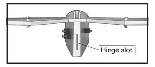
☐ 2) Glue the vertical fin in place using as same as techniques used to installing the horizontal fin.
