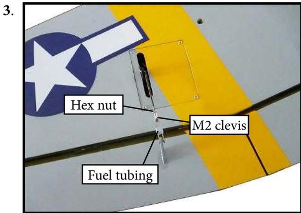
**INSTALLING THE FLAP PUSHROD**
