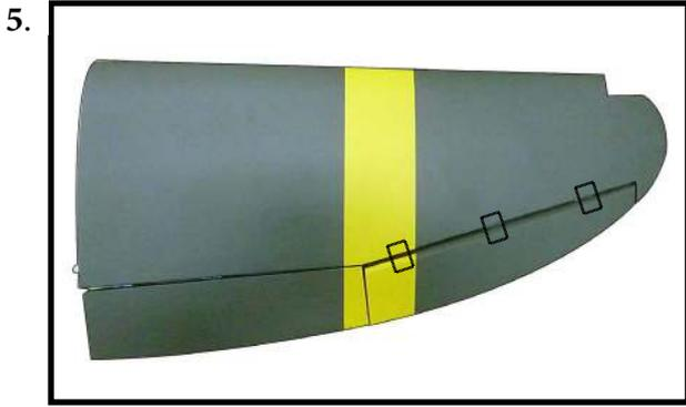
**Note:** Work the aileron up and down several times to "work in" the hinges and check for proper movement.
