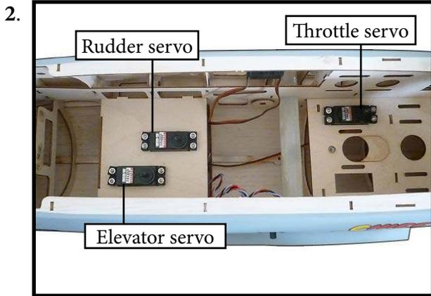
**THROTTLE SERVO ARM INSTALLATION**
