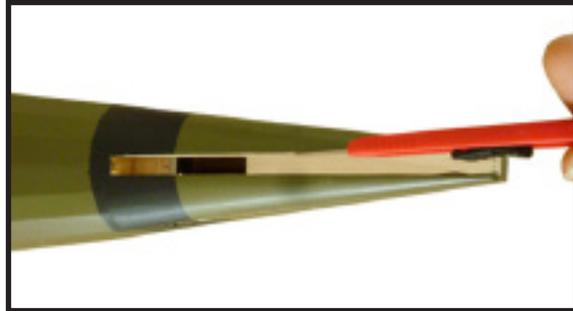
3) Slide the vertical stabilizer into the slot in the top of the fuselage. The rear edge of the stabilizer should be flush with the rear edge of the fuselage and the lower rudder hinge should engage the precut hinge slot in the lower fuselage. The bottom edge of the stabilizer should also be firmly pushed against the top of the horizontal stabilizer.
