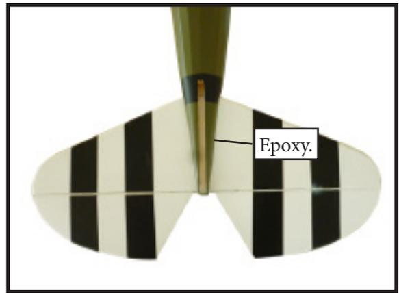
4) Slide the vertical stabilizer back in place. Using a triangle, check to ensure that the vertical stabilizer is aligned  $90^\circ$  to the horizontal stabilizer.
