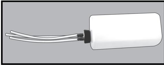
**!** *You should mark which tube is the vent and which is the fuel pickup when you attach fuel tubing to the tubes in the stopper. Once the tank is installed inside the fuselage, it may be difficult to determine which is which.*
