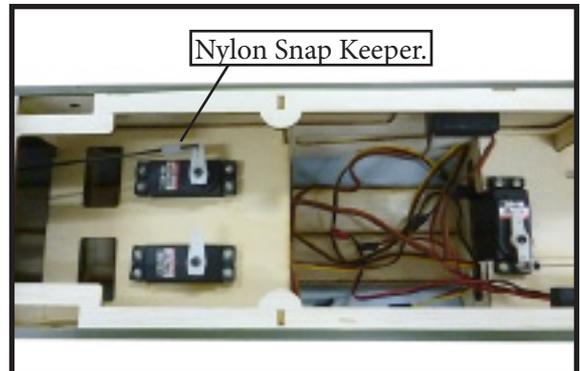
**RUDDER PUSHROD INSTALLATION.**
