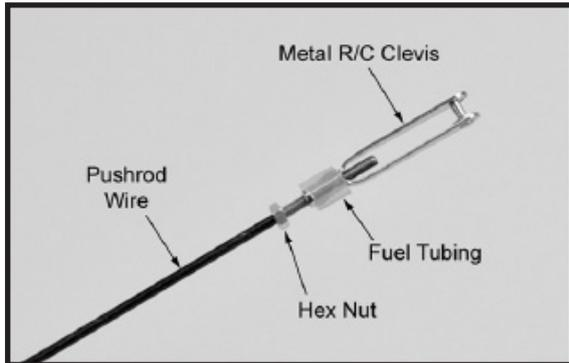
Use a felt tip pen to mark the wire where it crosses the hole. Use a pair of pliers to put a sharp 90-degree bend in the wire at the mark.
