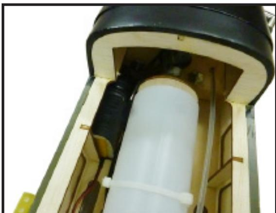
8) Use balsa block to hold in place the fuel tank with C/A glue to secure the fuel tank inside the fuselage.
