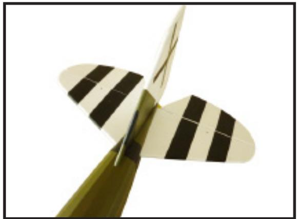
5) When you are sure that everything is aligned correctly, mix up a generous amount of Flash 30 Minute Epoxy. Apply a thin layer to the mounting slot and to bottom of the vertical stabilizer mounting area. Apply epoxy to the bottom and top edges of the filler block and to the lower hinge also. Set the stabilizer in place and realign. Double check all of your measurements once more before the epoxy cures.
