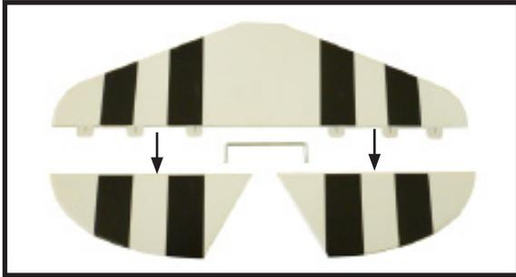
2) Carefully remove the elevator from one of the horizontal stabilizer panels. Note the position of the hinges.
