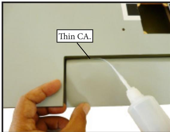
5) Turn the wing panel over and deflect the aileron in the opposite direction from the opposite side. Apply thin C/A glue to each hinge, making sure that the C/A penetrates into both the aileron and wing panel.
