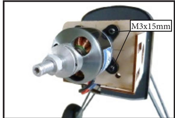
4) Attach the motor to the front of the electric motor box using four 4mm blind nut, four M3x15mm hex head bolts to secure the motor. Please see picture shown.
