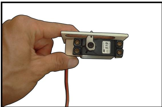
2) Use drill bit in a pin vise to drill the mounting holes in the blocks.
