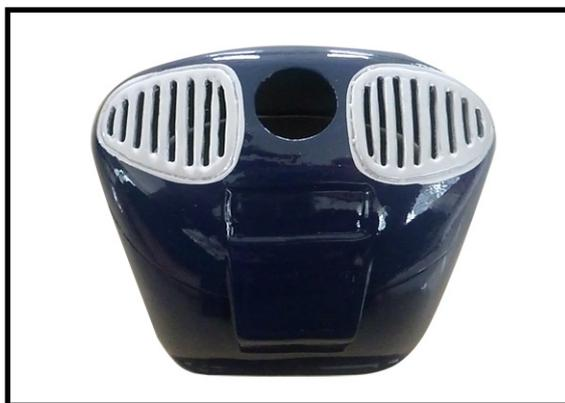
2) While keeping the back edge of the cowl flush with the marks, align the front of the cowl with the crankshaft of the engine. The front of the cowl should be positioned so the crankshaft is in nearly the middle of the cowl opening. Use the spinner backplate as a guide. Hold the cowl firmly in place using pieces of masking tape.
