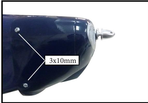
3) Install the muffler and muffler extension onto the engine and make the cutout in the cowl for muffler clearance. Connect the fuel and pressure lines to the carburetor, muffler and fuel filler valve. Secure the cowl to fuselage using the M3x10mm screws.
