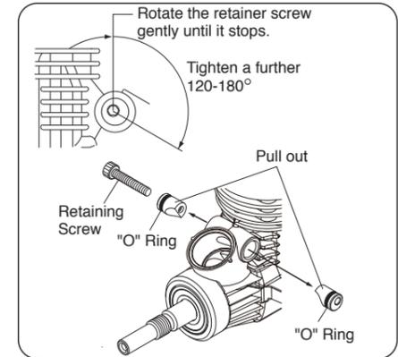
1. Loosen the retainer screw, rotate the carburetor to its correct position and make sure that it is pressed well down into the intake boss, compressing the rubber gasket, before retightening screw.
