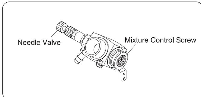
REALIGNMENT OF MIXTURE CONTROL VALVE
