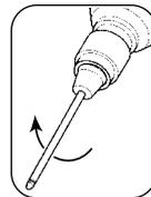
**5. Inserting the starter shaft**
