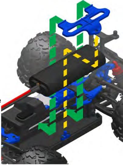
**Note:** Always unplug the battery and remove from the model after use.
