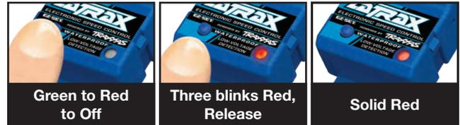
**i** Patent-Pending Training Mode (Profile #3) reduces forward and reverse throttle by 50%. Training Mode is provided to reduce the power output, allowing beginning drivers to better control the model. As driving skills improve, simply change to Sport or Race Mode for full-power operation.
