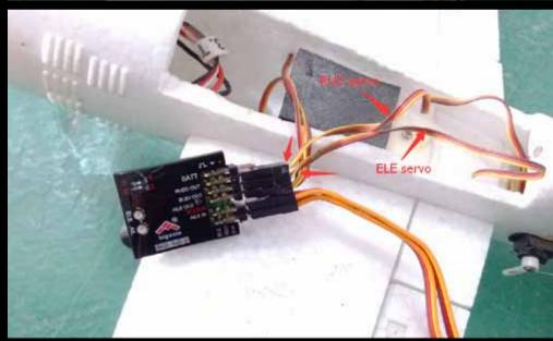
Connect receiver with motor
