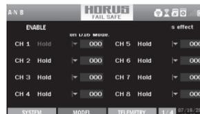
• No Pulse: on loss of signal the receiver produces no pulses on any channel. To use this type, select it in the menu and wait 9 seconds for the failsafe to take effect.
