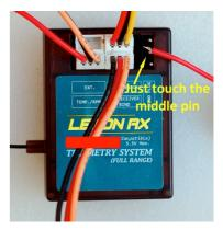
2. **Receiver Voltage**: Again briefly touch the RPM wire to the middle pin of the bind connector. The red LED should start to flash. Turn the pot until the receiver voltage shown on the transmitter screen agrees with the value measured using an accurate voltmeter.
