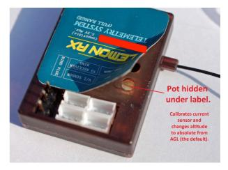
Expose the pot/switch and have a small screwdriver ready to adjust it.
