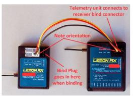
And here is the same setup for a Lemon 7channel stabilized receiver.
