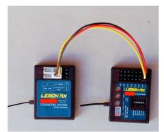
Here is what it looks like with an Orange RX3SM. Although the servo ports on this receiver are Molex 1.25mm pitch Picoblade connectors, the bind connector is a standard 0.1" header.
