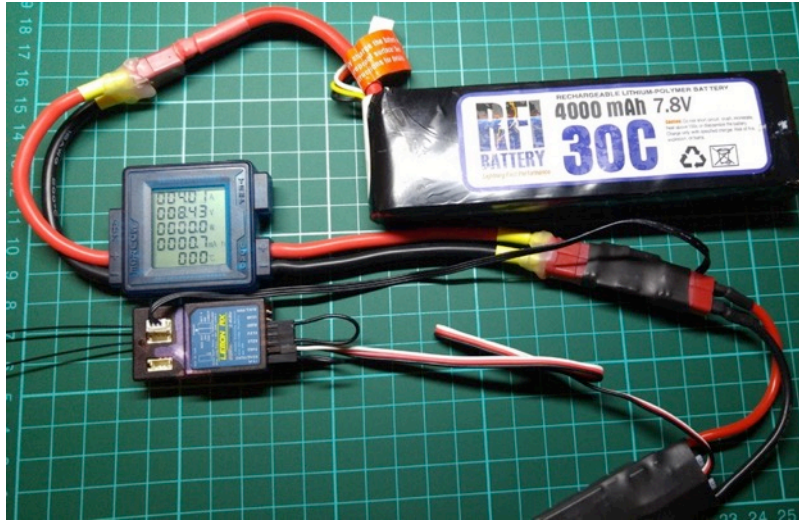
Figure 3.5 – V/I sensor calibrated at 8.4V and 4A, as shown on the Wattmeter.
