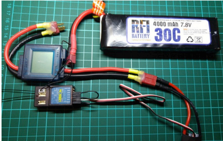
Figure 3.2 – Voltage sensor wire connected to battery V+. First bind plug is in normal vertical location, second is inserted horizontally between the top (signal) pins of Aileron and Rudder channels. The device with a screen is a Wattmeter, which measures voltage and current and is used to confirm the battery voltage.
