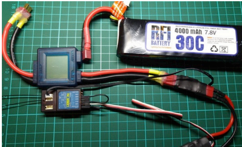
Figure 3.4 – V/I sensor connected to battery V+ with two bind plugs inserted. The device with a screen is a Wattmeter to confirm the actual battery voltage and current.
