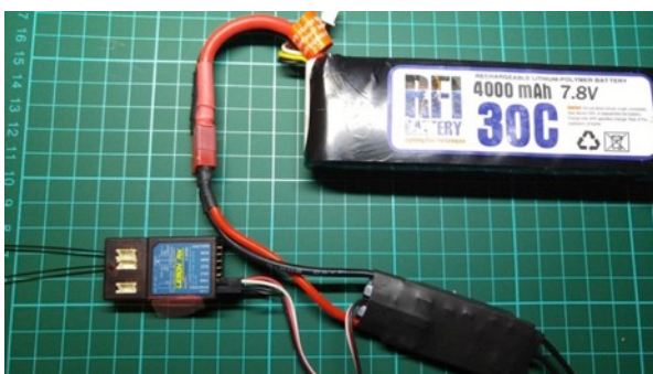
Figure 2.2 – Solid red light on bottom of receiver indicates successful binding.
