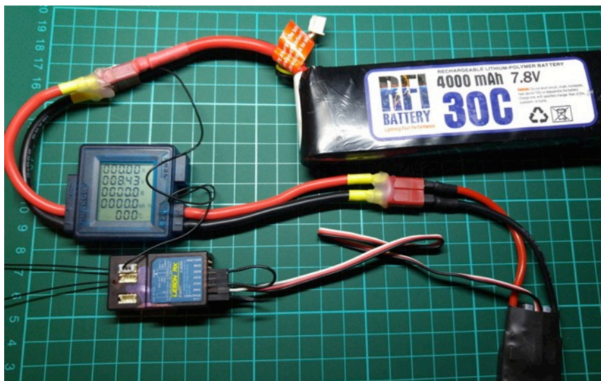
Figure 3.3 – Battery now plugged in. Note voltage sensor wire. Voltage sensor is calibrated at 8.43V, as shown on Wattmeter.
