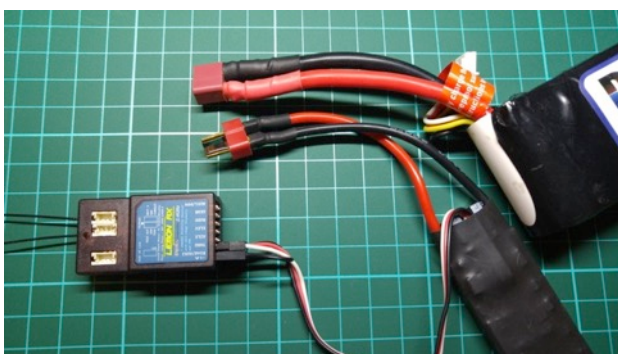
Figure 2.1 – Bind plug inserted with power disconnected.
