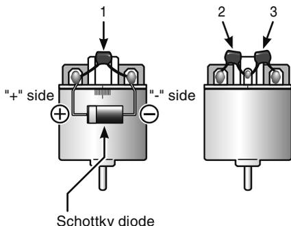
Motors with no suppressor capacitors, or inadequate suppression, may cause the receiver to malfunction. Always solder the capacitors supplied to your motor. The Schottky diode improves the efficiency of the speed control / motor combination and provides extra protection to the brake FETs. The white ring must always face the positive side.
