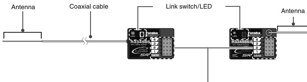
\*R314SB-E has no external antenna. LED / Link switch and connector part are the same as R314SB.
