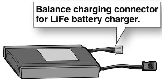
**LiFe battery is removed from the transmitter.**
