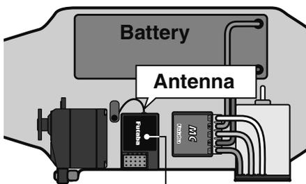
Install the receiver as far away as possible from the battery, motor controller, motor, silicon cord and other noise sources. Keep it away from the antenna wire, in particular. The example in the figure is for R334SBS. The R334SBS-E places the antenna holder on the top of the case.
