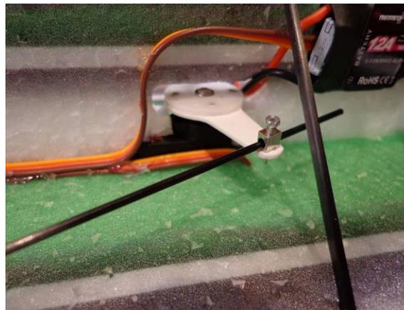
Install the set screw. Be very careful, there are not many threads and it is easy to cross thread. Only snug up, a ton of pressure is not needed. Make sure the servo is centered
