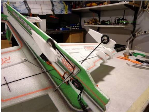
Repeat for the other wheel pant, double check that they are lined up and if having used Welders let dry for a bit
