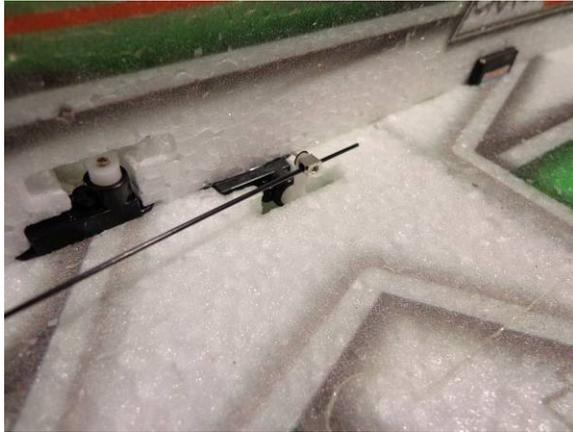
Slide the free end thru the hole in the elevator servo's adjustable link. Don't worry about any extra at this time
