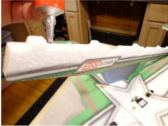
Also apply a thin layer to the upper vertical fuselage piece. Note avoid the areas that come into contact with the servos
