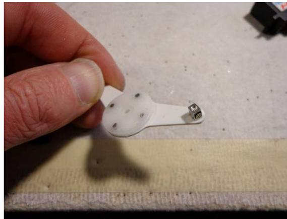
Install the adjustable links from the side shown, use the same technique as with the tail servo horns
