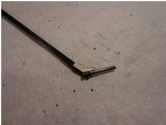
Again with a drop of medium CA attach the stub axle as shown and hit with kicker
