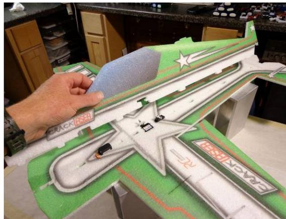
As with the bottom fuselage, check the fit of the upper fuselage and make additional cuts as needed
