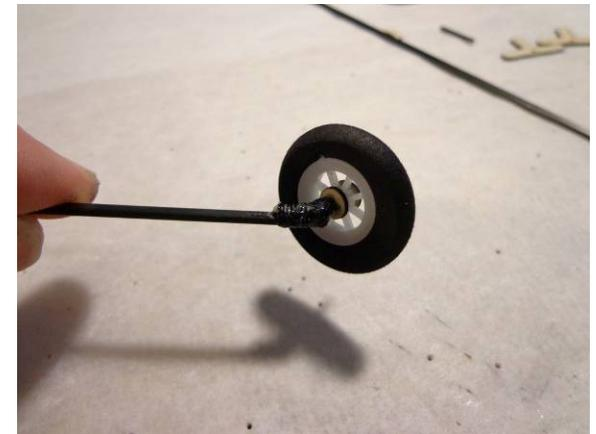
Wrap the thread as shown and soak with thin CA and hit with Kicker. Install the inside washer and also CA, slide on the wheel and outside washer
