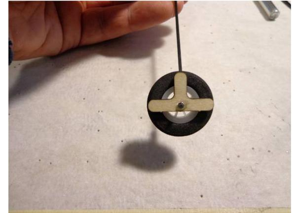
Align the brace as shown in the picture above and then glue from the outside with medium CA and Kicker
