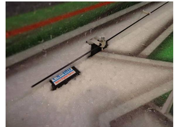
Do the same for the rudder push rod, again not a lot of pressure and make sure the servo and control surface are centered
