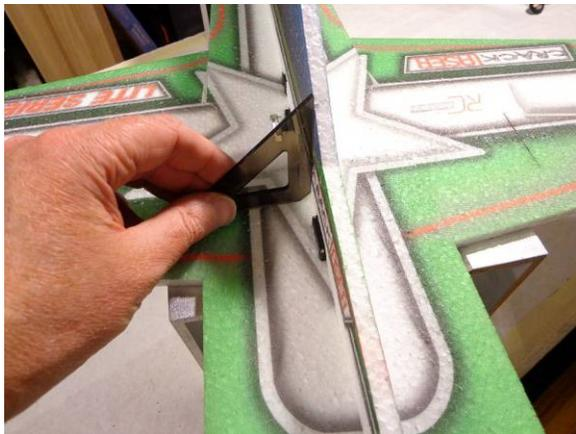
While the glue is still wet, make any adjustments as needed for squareness. Let the glue set up for 15 or 20 minutes before handling
