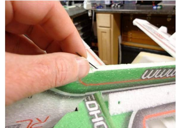
With the scrap from the previous step, poke (and glue) one of the skinny pieces into the tail as shown to help keep the rudder off the ground
