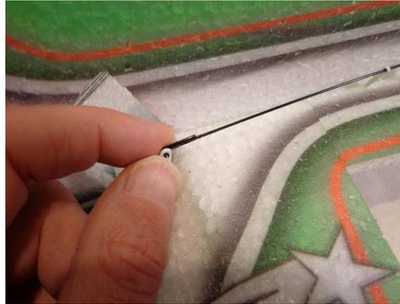
Snap the Snap Link into the elevator control horn. For this model snapping from the inside will yield a straighter line for the control rods
