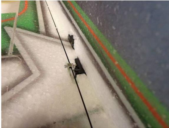
Repeat for the elevator push rod. Servo and control surface centered when snugging up the set screw
