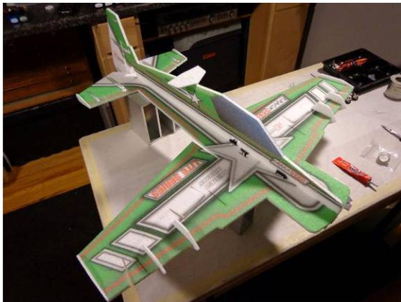
Skim coat the ends of all the hinge lines as well. Wait a couple minutes and attach the tape, the longer pieces are for the motor mount and the others ones the hinge lines
