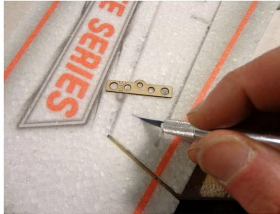
Clean out the slots in the wing where the ribs will be installed. Note that the ribs are the same width as the wing thickness
