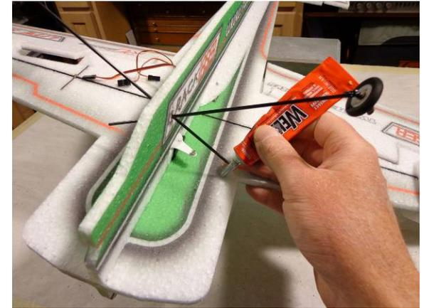
Flip the plane back over, remove the ends of the struts from the Horz Fuse section, put some glue in the hole and re-install
