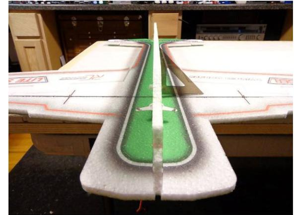
Make sure pieces are true to each other, and fully seated to one another, apply pressure for approx 15 min. before moving
