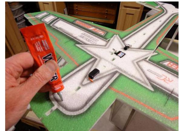
Apply a thin layer of Welders to the mating surface as shown
