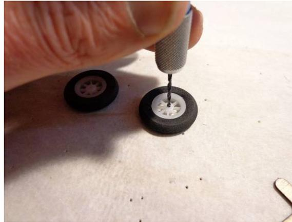
Drill out the center of the wheels to fit the small axle stubs, should be approx 1/16" diameter
