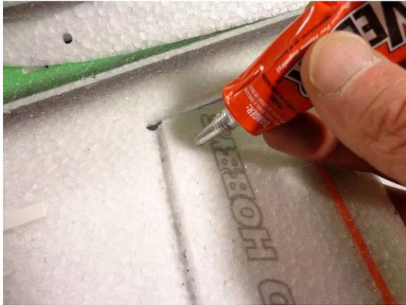
With the tip of the Welder's tube, squeeze some glue into the slit, and put a skim coat of glue on the horn
