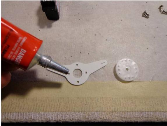
Apply a thin layer of Welders to the differential horn as shown above
