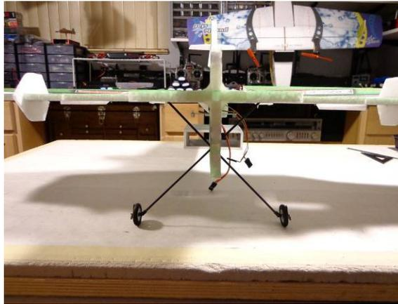
Adjust the position of the struts where they cross the fuselage to ensure that once glued in that the plane will sit level
