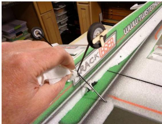
Once you are sure there is plenty of glue in and around the struts where they cross thru the fuselage, wipe away any extra glue
