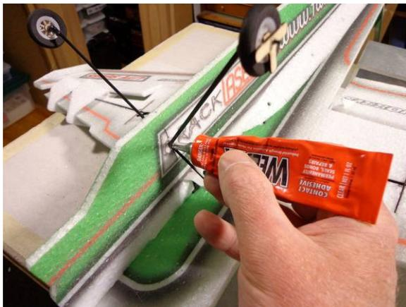
Squeeze some Welders into the area of the fuselage where the struts cross. Do this from both sides, don't worry about extra glue at the moment
