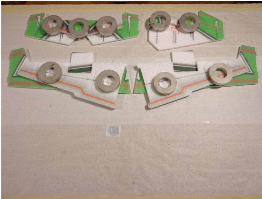
Locate the hinged items as shown above, bend them back onto each other as shown and let set for an hour or so. This process will help to loosen up the movement of the control surface, and is necessary to prevent servo damage.
