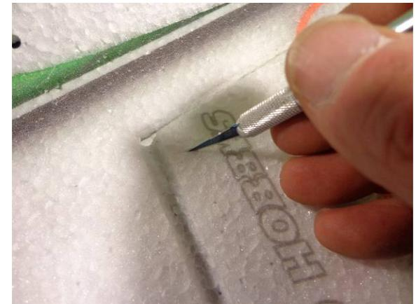
Using the pre-cut slots for the aileron horns as a guide, increase the depth so the horns will fit flush to the bottom surface
