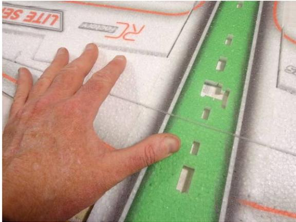
Once the glue has tacked up, bring all the pieces together. Note that all the tabs and slots should line up and parts are "keyed" for proper orientation
