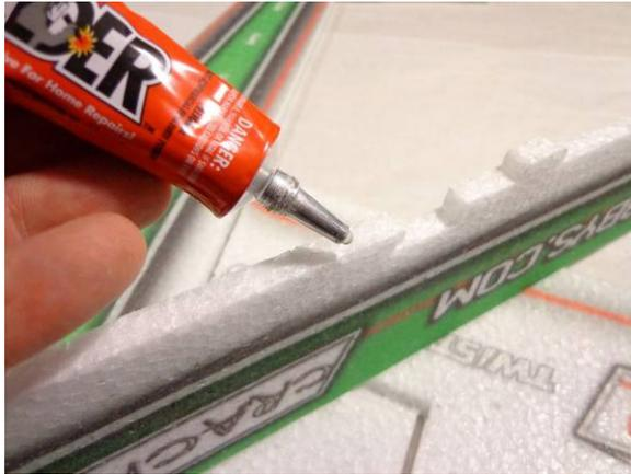
Immediately apply a thin layer to the mating surfaces of the lower vertical fuselage....
