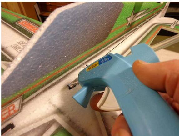
With Low Temp Hot Glue (or Welders as seen in the next picture) lay a bead of glue down in two places on each servo, this should be enough to hold them in place
