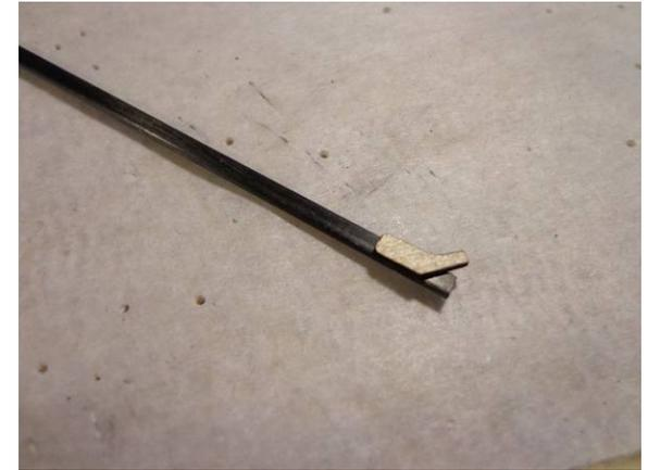
With a drop of medium CA join the rectangle carbon strut with the small wood piece as shown.
