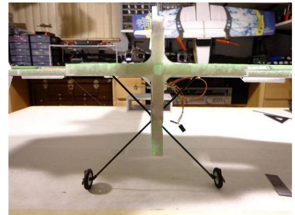
Flip the airframe back onto it's wheels and adjust so that it is level again like when the dry fit was done. Flip back over so the struts are facing up and let them dry
