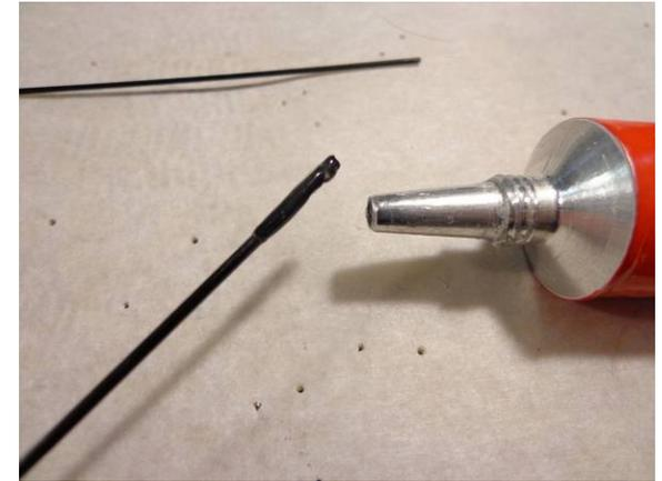
Pull the rod out and check that you have a nice even coat of glue as shown, if not, repeat the process
