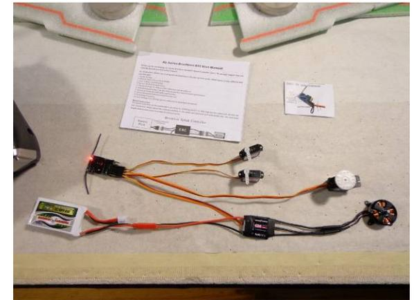
Hook up the entire electronics system as shown. Mount and center the control horns and servos as shown. Test for proper operation of all items
