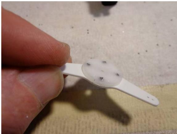
Trim off the extra screw length with some side cutters and grind smooth with a motor tool or hand file
