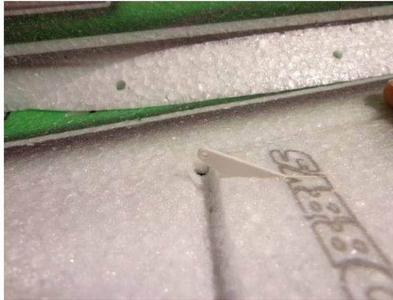
Install the aileron horn so that it is flush with the under side of the wing, and so that the hole is in line with the pivot point of the control surface
