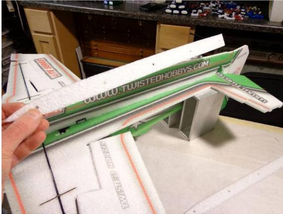
.... position the truss in place and then remove immediately. This transfers some of the glue... let it tack up then install
