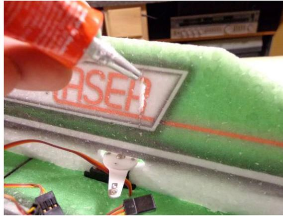
Squeeze some Welders into the upper and lower slits ONLY. Keep the center area of the opening free of glue at this time
