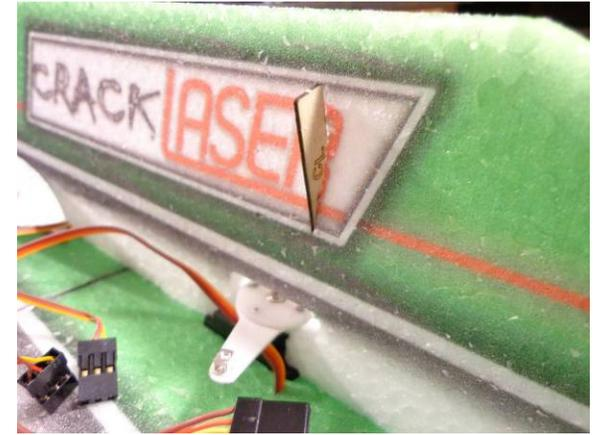
Slide the bulkhead into position and make flush with both sides of the fuselage
