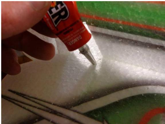
Back to the horns... Do the same thing with the slot on the elevator, squeeze some glue in and apply a skim coat of glue to the mating area of the horn
