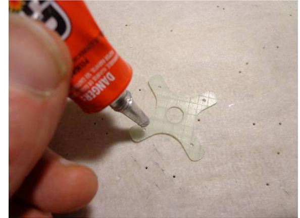
Motor mount is next... roughen up the glue side of the mount and coat with a medium amount of Welders and let tack up.
