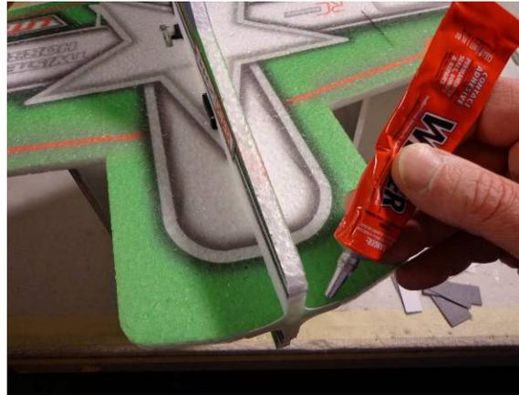
Apply a small bead of Welders directly behind the motor mount arms, top and bottom, left and right sides.....
