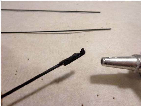
Attach a snap link as shown. Notice that the snap link has a "saddled" area, this should be where you rest the control rod
