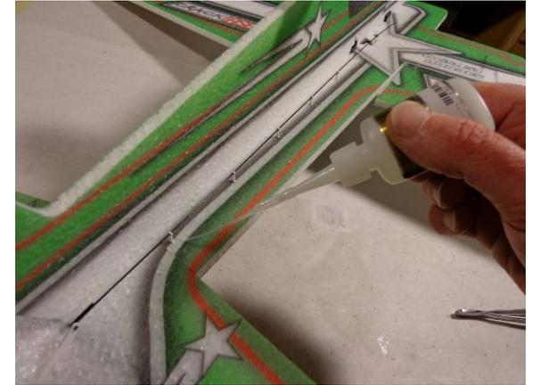
Locate the precut holes for the guides and install the base of the guides into each hole. Align them straight and then apply a drop of CA at the base of each
