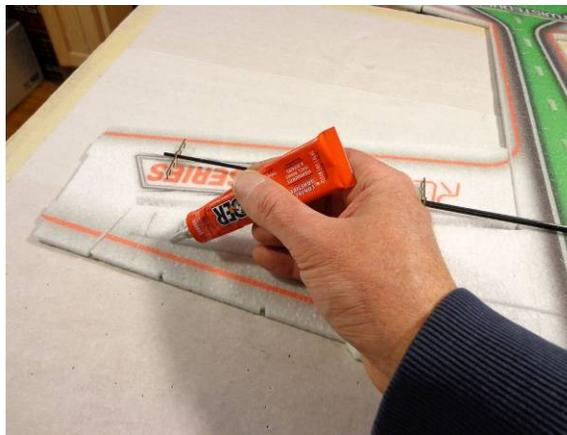
Once you are happy with the dry fit, remove the spar/rib assembly and fill all the appropriate slots in the wing with Welders
