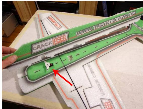
Install the aileron servo (no glue) as shown and test fit the bottom section of the fuselage, it may need to be trimmed a little around the aileron servo.
