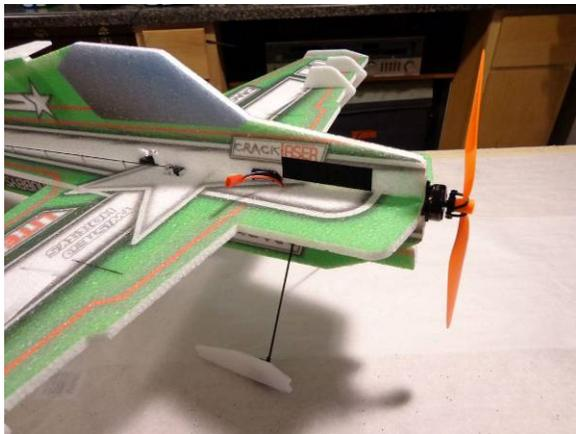
With the TH power combos and 2s/360 battery, location of the battery will be somewhere directly in front of the aileron servo. It is best to use velcro and fly the model before cutting a hole
