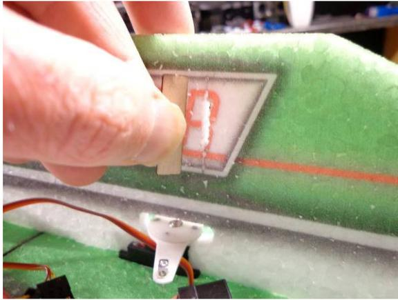
While holding the small rectangle wood bulkhead up for reference, slit either end of the opening so the bulkhead can install in the center of the opening
