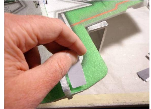
... spread the beads out to a skim coat thickness. This is the area you will apply the tape to. The Welders skim coat will help the tape stick.
