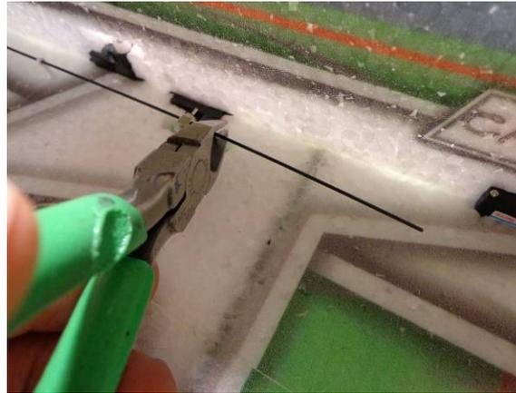
Trim all the control rods so there is only about 1/4" beyond the servo horn. Keep the longest piece of the tail rods to make a tail skid
