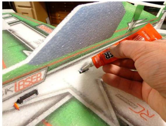
If deciding to use Welders instead of hot glue, do three or four "dabs" in two different places of each servo
