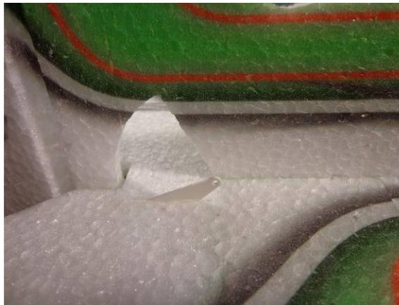
Install the horn from the TOP side of the elevator, and make sure the hole in the horn is in line with the pivot point of the elevator
