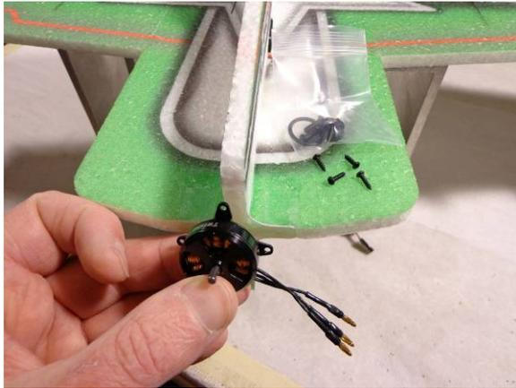
Locate your motor and its mounting hardware. Install with the wires facing the side in which the ESC will be installed on to
