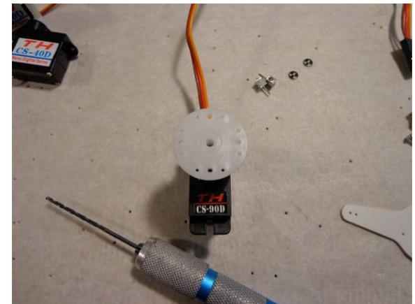
With the servo centered, mount the round servo horn for the aileron servo as shown and slightly enlarge the holes so that the mount screws will self tap
