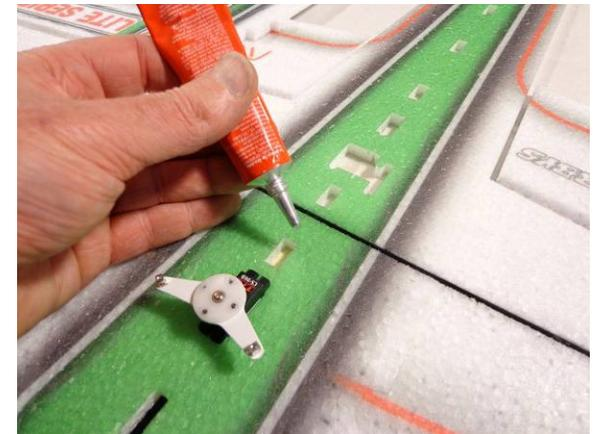
Once happy with the fit up apply a thin coat of Welders to the mating surface of the horizontal fuselage section
