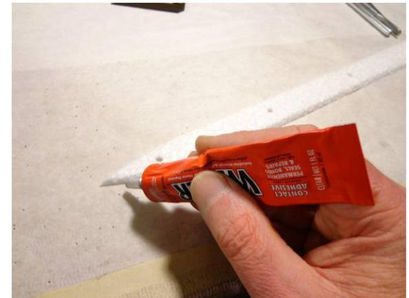
Tack up method will be used to attach the trusses. to do this apply a medium bead of Welders to the beveled area of the truss....
