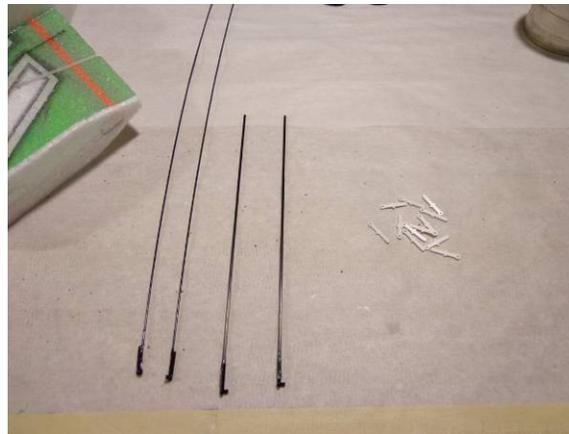
If it has been about 24 hours now since gluing the snap links on, grab the long ones and get ready to install the control rods for the tail surfaces
