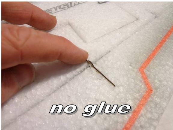
Check the fit of the ribs to the slot in the foam, with the exception of the humped area, the rib should sit flush with both the top and bottom surfaces
