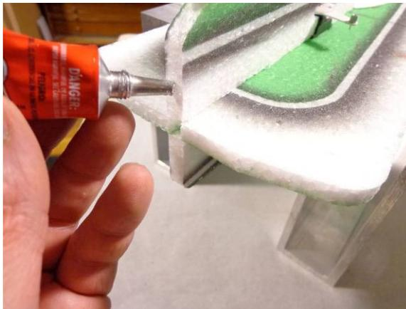
Apply a medium coat of Welders to the mating area of the fuselage nose and let tack up as well
