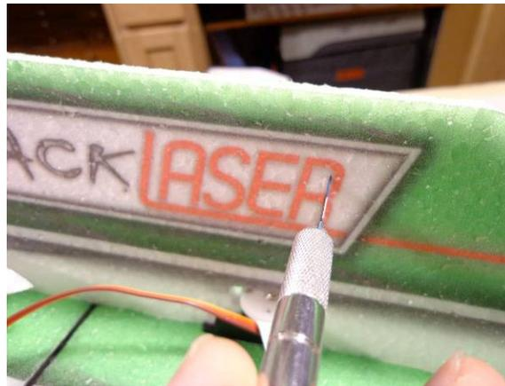
The next couple steps are for installing the landing gear if not wanting the gear, skip past them. Locate the holes and open up the area in between them
