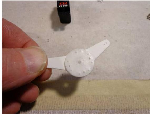
Install the Diff Horn from the **underside** of the stock servo horn as pictured, line up the holes between the two pieces
