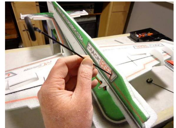
Slide one of the struts in from the left to the right. There is a small pre-cut hole in the horizontal fuselage piece that will receive the raw end
