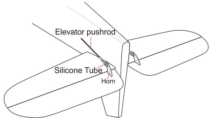
1) Using pliers, carefully make a 90 degree bend down at the mark made. Cut off the excess wire, leaving about 6mm beyond the bend.
