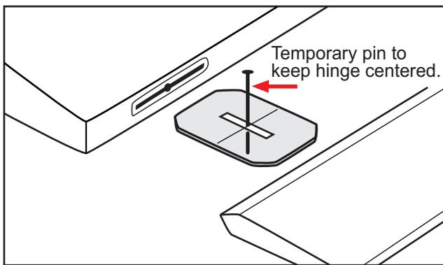
\* Apply drops of thin CA to the top and bottom of each hinge. Do not use CA accelerator. After the CA has fully hardened, test the hinges by pulling on the aileron.
