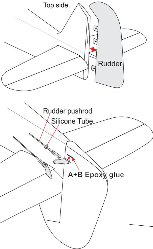
Control horn and linkages for Rudder are installed the same way as the Elevator before (see page 10).
