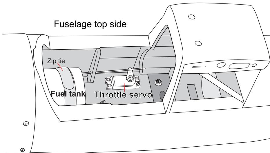
**INSTALLING THE THROTTLE PUSHROD**
