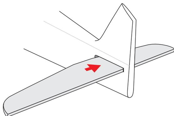
3) Check the fit of the horizontal stabilizer in its slot. Make sure the horizontal stabilizer is square and centered to the fuselage by taking measurements, but don't glue anything yet.
