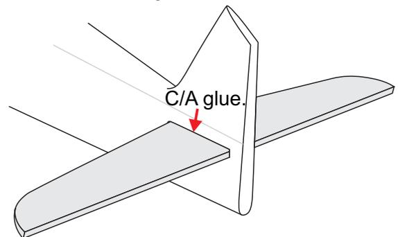
6) Hinges for Elevator are glued the same way as the aileron before (see page 4).
