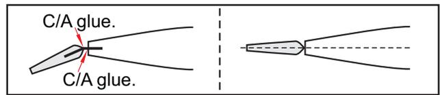
\* Secure nylon hinges with instant glue, being careful not to glue the wing and aileron together.
