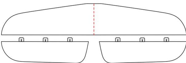
1) Using a modeling knife, carefully remove the film covering from the tail slots at the rear of the fuselage. Make sure that you do not remove any wood from the slots as this will affect the alignment of the tail.
