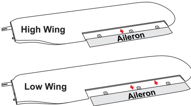
\* Test fit the ailerons to the wing with the hinges. If the hinges don't remain centered, stick a pin through the middle of the hinge to hold it in position.
