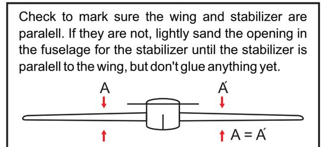
Check to make sure the wing and stabilizer are parallel. If they are not, lightly sand the opening in the fuselage for the stabilizer until the stabilizer is parallel to the wing, but don't glue anything yet.
