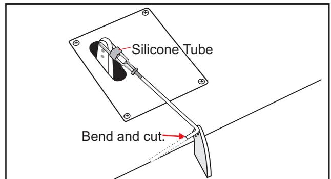
Insert the 90 degree bend down through the hole in the control horn. Install one nylon snap keeper over the wire to secure it to the control horn. Install the control horn retaining screw and remove the masking tape from the aileron.
