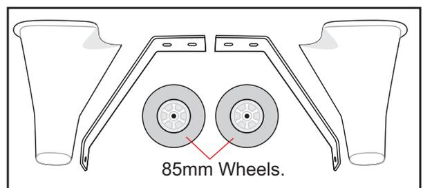
Secure the gear to the fuselage.
