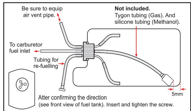
5) Test fit the stopper assembly into the tank. It may be necessary to remove some of the flashing around the tank opening using a modeling knife. If flashing is present, make sure none of it falls into the tank.
