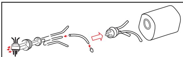
8) Feed three lines through the fuel tank compartment and through the pre-drilled hole in the firewall. Pull the lines out from behind the engine, while guiding the fuel tank into place. Push the fuel tank as far forward as possible, the front of the tank should just about touch the back of the firewall. Blow through one of the lines to ensure the fuel lines have not become kinked inside the fuel tank compartment. Air should flow through easily.
