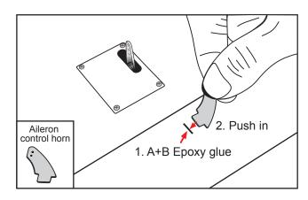
☐ 3) Repeat the procedure to install the control horn on the opposite aileron.
