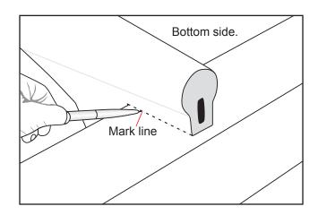
☐ 6) Remove the stabilizer. Using a modeling knife and ruler **CAREFULLY** cut 1mm **inside** the marked lines. Remove the covering from the top and the bottom of the tail plane.
