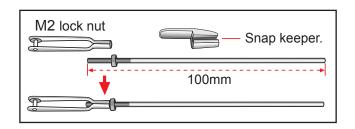
Using pliers, carefully make a 90 degree bend down at the mark made. Cut off the excess wire, leaving about 6mm beyond the blend.
