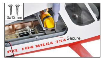
Position the canopy so the rear frame on the canopy is aligned with the fuselage. Use canopy glue to secure the canopy to the fuselage. Use low-tack tape to hold the canopy in position until the glue fully cures. Wrap the tape completely around the fuselage.
