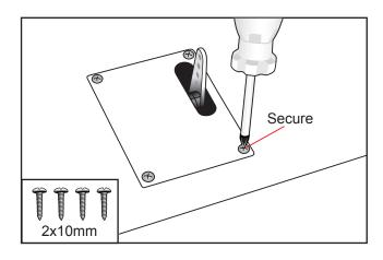
☐ 5) Repeat the procedure to install the aileron servos in the opposite wing half.
