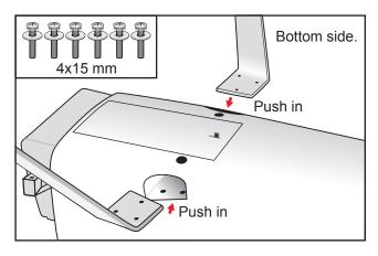
Secure the gear to the fuselage.
