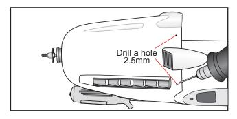
Drill four 2.5mm pilot holes through both the cowl and the side edges of the firewall. Using a 3mm drill bit, enlarge the four holes in the cowling.
