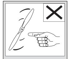
**THE PROPELLER IS DANGEROUS.** Keep fingers, clothing (ties, shirt sleeves, scarves) or any other loose objects that could be caught or drawn in, away from the propeller. Take care at **ALL** times.
