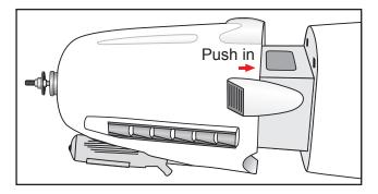
□ 2) While keeping the back edge of the cowl flush with the marks, align the front of the cowl with the crankshaft of the engine. The front of the cowl should be positioned so the crankshaft is in **nearly** the middle of the cowl opening. Hold the cowl firmly in place using pieces of masking tape.
