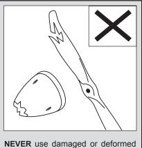
**NEVER** use damaged or deformed propellers or spinners.
