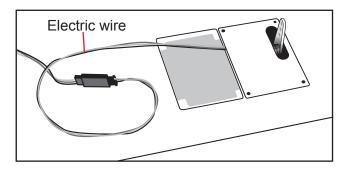
□ 4) Place the servo into the servo tray. Center the servo within the tray and drill 1.5mm pilot holes through the block of wood for each of the four mounting screws provided with the servo.
