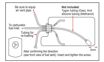
$\Box$  5) Test fit the stopper assembly into the tank. It may be necessary to remove some of the flashing around the tank opening using a modeling knife. If flashing is present, make sure none of it falls into the tank.
