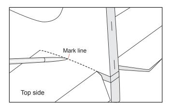
□ 6) Remove the stabilizer. Using the lines you just drew as a guide, carefully remove the covering from between them on the top and bottom of the tail plane using a modeling knife.
