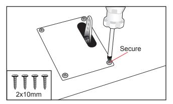
**5)** Repeat the procedure to install the aileron servos in the opposite wing half.
