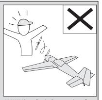
**ALWAYS** adjust the engine from behind the propeller, and do not allow any part of your body to be in line with the propeller.
