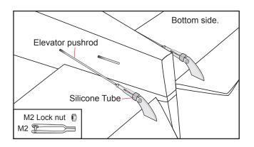
□ 1) Using pliers, carefully make a 90 degree bend down at the mark made. Cut off the excess wire, leaving about 6mm beyond the blend.
