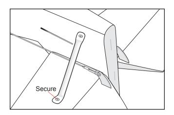
Repeat the procedure to install the other horizontal stabilizer struts.
