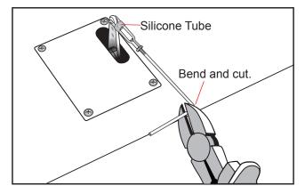
Insert the 90 degree bend down through the hole in the control horn. Install one nylon snap keeper over the wire to secure it to the control horn. Install the control horn retaining screw and remove the masking tape from the aileron.
