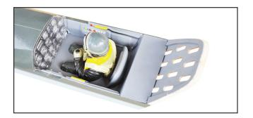
Position the canopy so the rear frame on the canopy is aligned with the rear edge of the cockpit opening. Use canopy glue to secure the canopy to the canopy hatch. Use low-tack tape to hold the canopy in position until the glue fully cures. Wrap the tape completely around the canopy hatch, as the tape does not stick well to the covering. We used balsa sticks to hold the lower edges of the canopy tightly against the canopy hatch.
