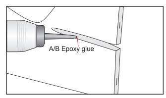
After the epoxy has fully cured, remove the masking tape or T-pins used to hold the stabilizer in place and carefully inspect the glue joints. Use more epoxy to fill in any gaps that may exits that were not filled previously and clean up the excess using a paper towel and rubbing alcohol.
