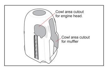
$\Box$  1) Slide the fiberglass cowl over the engine and line up the back edge of the cowl with the marks you made on the fuselage.
