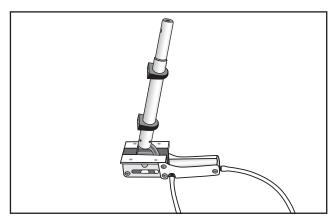
Place the retract to the wing and pull out the air tube through the wing section.
