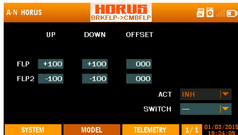
Overview of the brakeflap->camberflap menu screen
