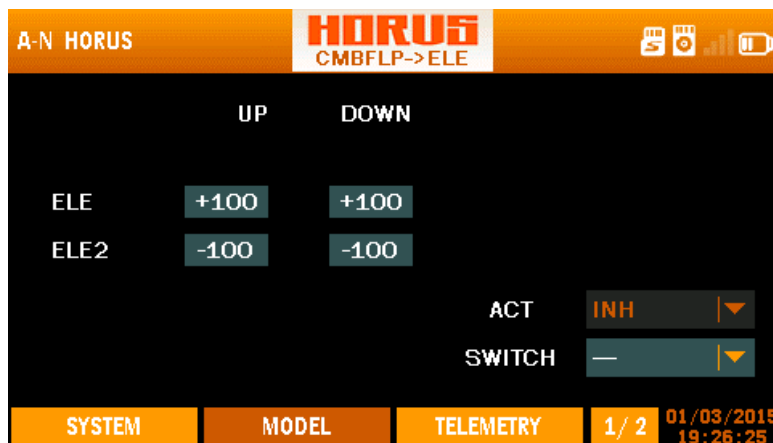
Overview of the camberflap->elevator 1/2 menu screen
