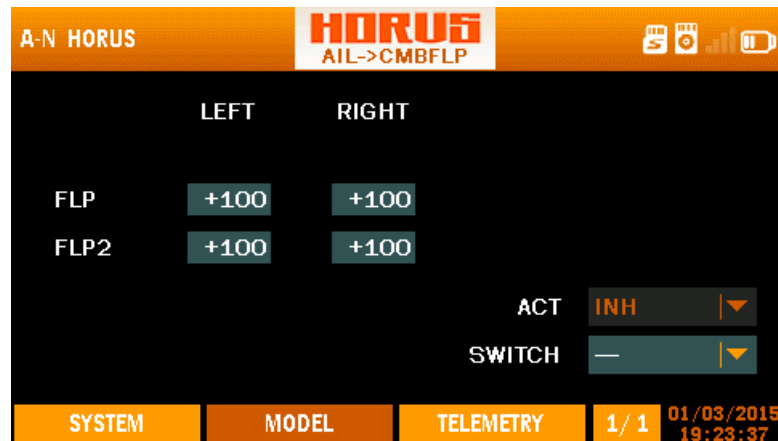
Overview of the aileron->camberflap menu screen
