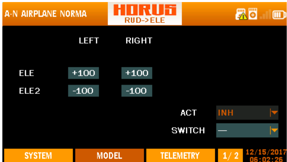
Overview of the rudder->elevator 2/2 menu screen
